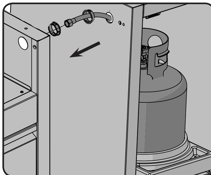
The gas connection of the Mirage series grills is at the left of the control panel. Placing the tank enclosure cabinet to the left of the unit cabinet will make for easier gas piping. Knockouts have been punched in the sides and back panels to provide easy routing of gas or electrical piping. Once the knockout has been removed a bushing must be installed to prevent the gas or electrical line being cut on the edge of the hole. Gas piping and installation must be done by a qualified gas installer.
