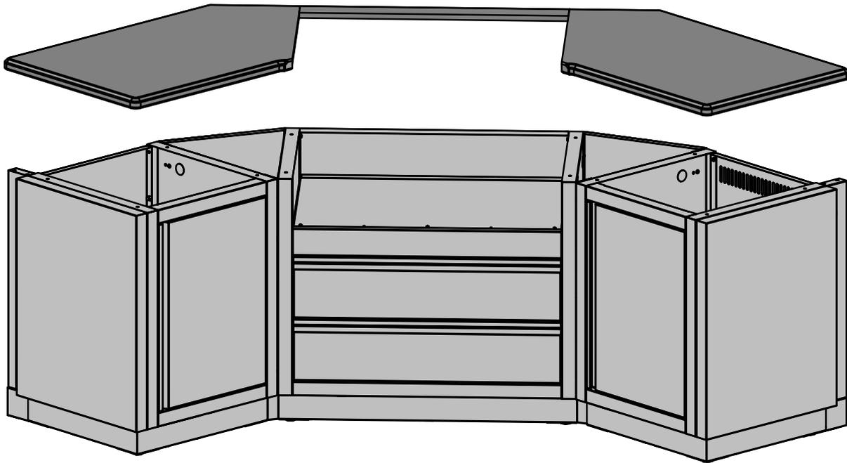
COUNTERTOP TO BE FASTENED AS PER MANUFACTURER'S INSTRUCTIONS. HOLES HAVE BEEN PLACED ON THE TOP FLANGE OF THE SIDE PANELS TO ALLOW FOR FASTENERS.
