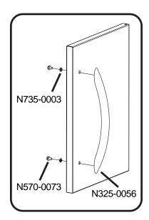
The door handle is mounted inside the door for shipping purposes. It must be removed and mounted to the outside surface of the door. Slots are provided in the door skin to ensure proper alignment of the top edges of the handles on each door.
