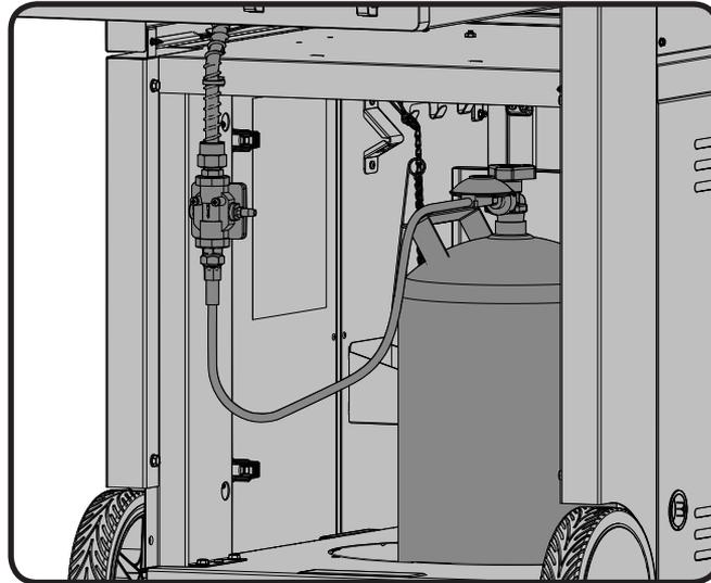
All cylinders 7kg or larger must be placed outside the enclosure (under the right side shelf) on level ground. The hose assembly must be routed through the knock out hole in the right side panel.
