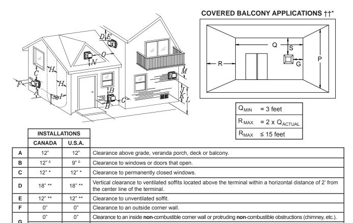
Clearance to an inside combustible corner wall or protruding combustible obstructions (vent chase, etc.).
