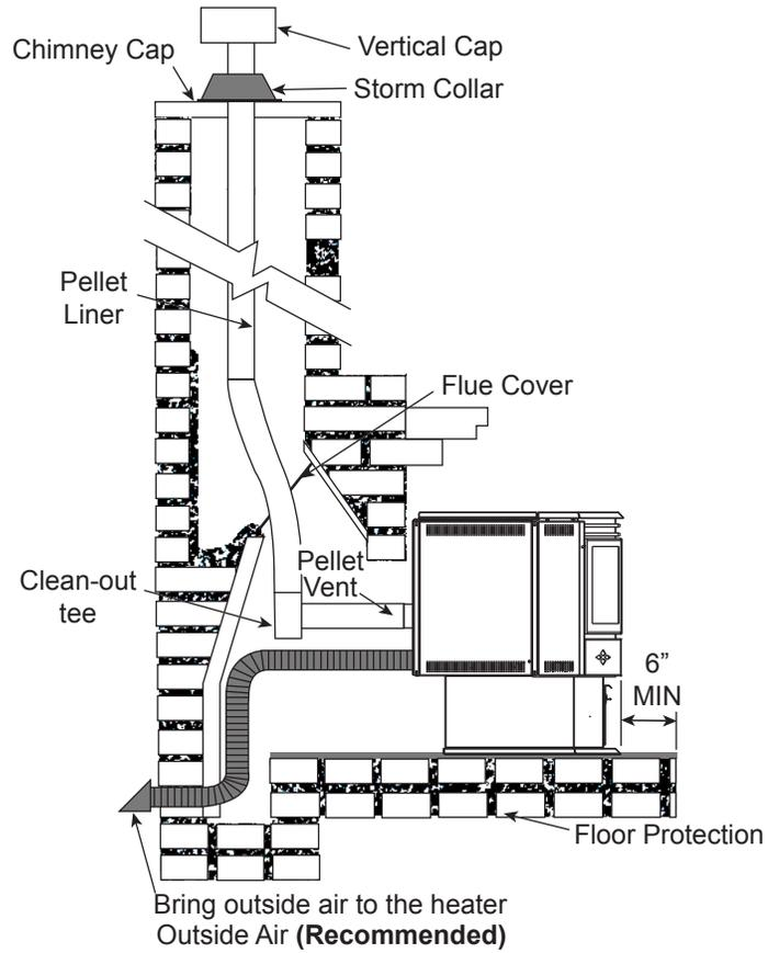
For installation instructions, see manufacturer's installation instructions and "typical existing masonry" section.
