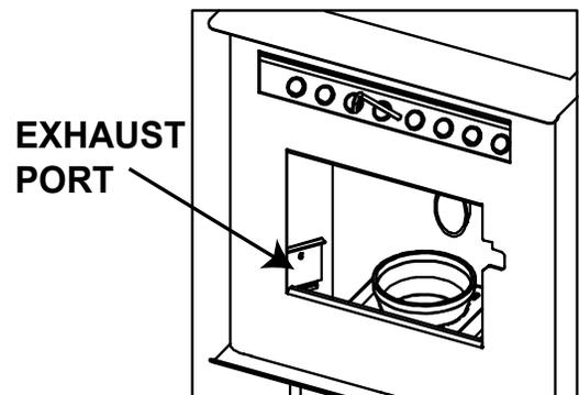
Once clean, replace the exhaust port doors and secure with the screws.
