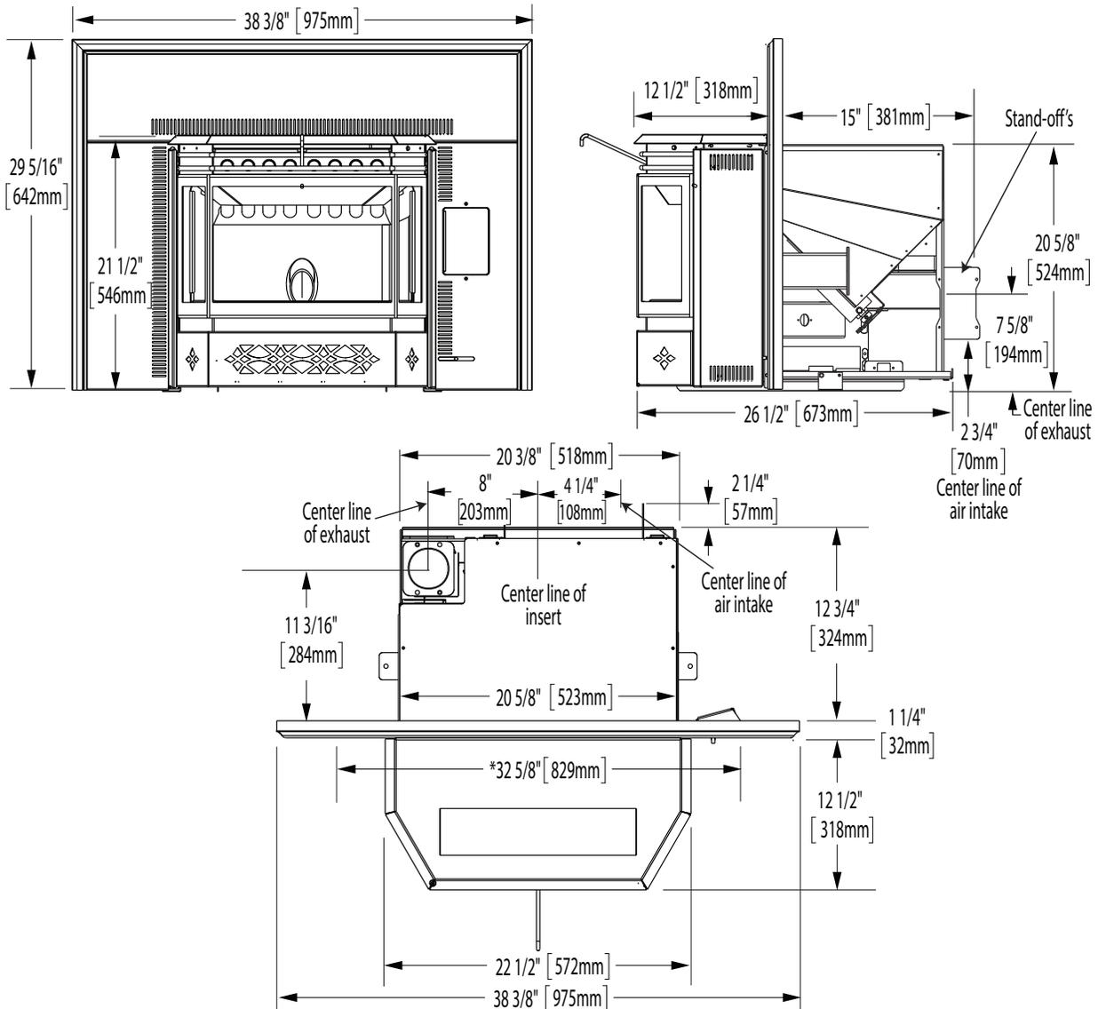
\*In order to install flashing flush to a finished wall and centered within the opening, the front opening of the fireplace or enclosure must be this wide.
