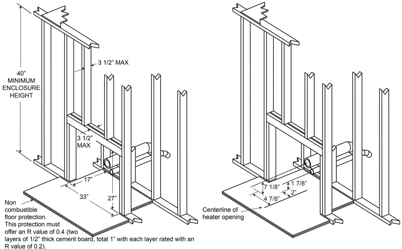
For temperature requirements, the enclosure space around and above the heater must be left unobstructed.
