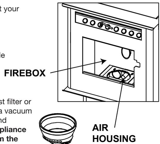
Re-install the burn pot ensuring it sits level in the appliance. Also must ensure the ignitor and the burn pot
