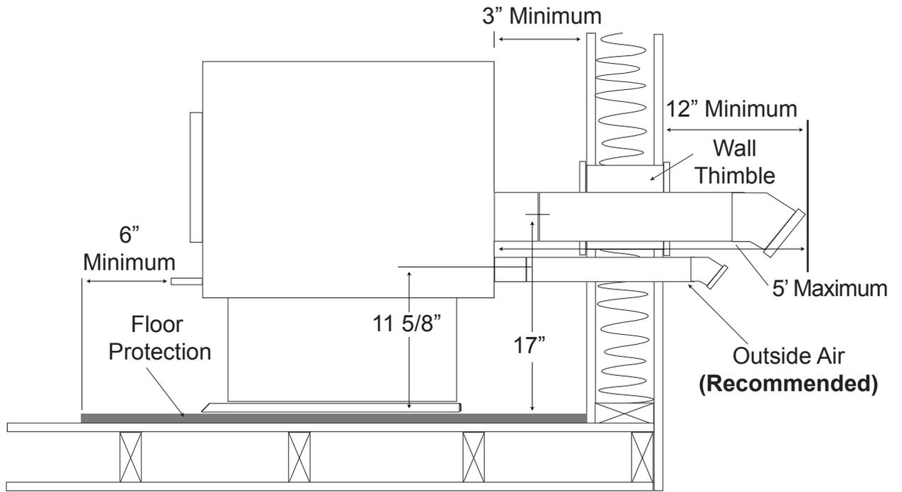
4.5.2 through the wall with vertical rise / horizontal termination
