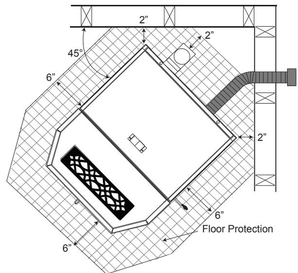
**NOTE:** If interior vertical pellet vent is used, the clearance to the back wall is determined by the upward-turning elbow or "Tee". It will vary in depth depending on the brand of pellet vent used (it is approximately 5" (127mm)). Before placing the appliance, connect the elbow or "Tee" and allow for the minimum 3" (76mm) clearance to the combustible wall.
