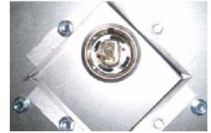
**When re-assembling the light assembly, care must be taken. “Light Leakage” from above the cast doors may be noticed. The holes in the lamp housing are necessary for ventilation and must not be covered.**
