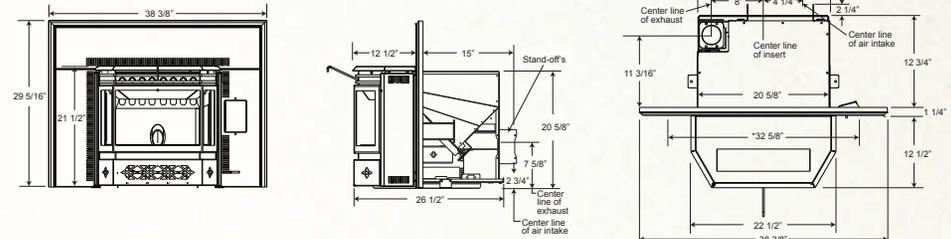
\*In order to install flashing flush to a finished wall and centered within the opening the front opening of the fireplace or enclosure must be this wide.
