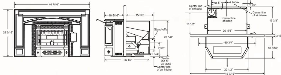
\*In order to install flashing flush to a finished wall and centered within the opening the front opening of the fireplace or enclosure must be this wide.
