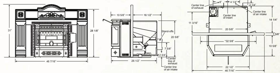
\*In order to install flashing flush to a finished wall and centered within the opening the front opening of the fireplace or enclosure must be this wide.
