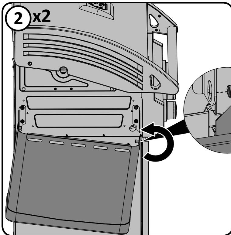
Bend shelf open slightly to insert second pin into bracket.
