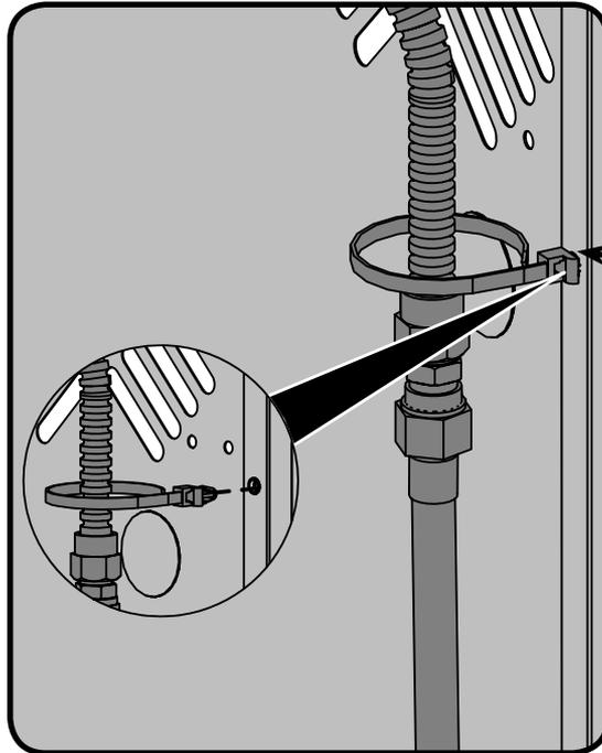
Clip hose to side panel using hose retainer clip supplied.
