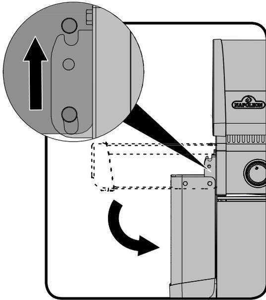
Push down and engage top pins to lock shelf in place.
