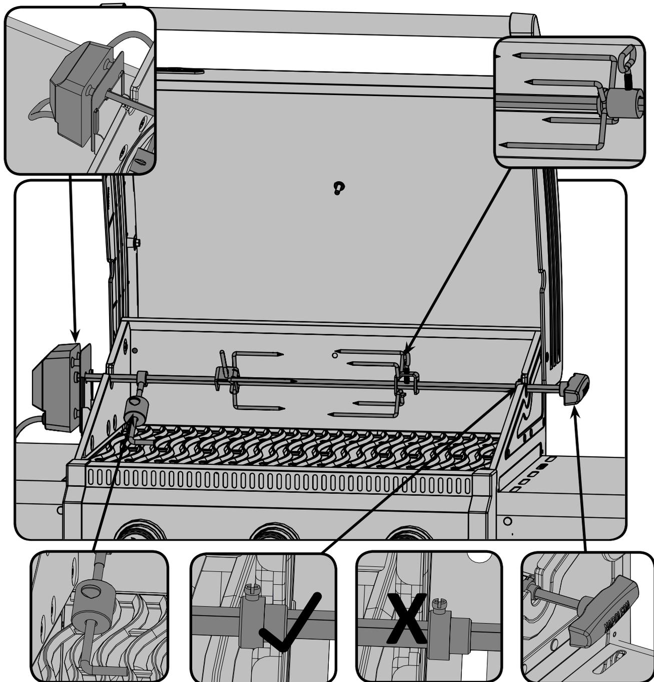
**Ensure stop bushing is tightened on the inside of hood casting.**
