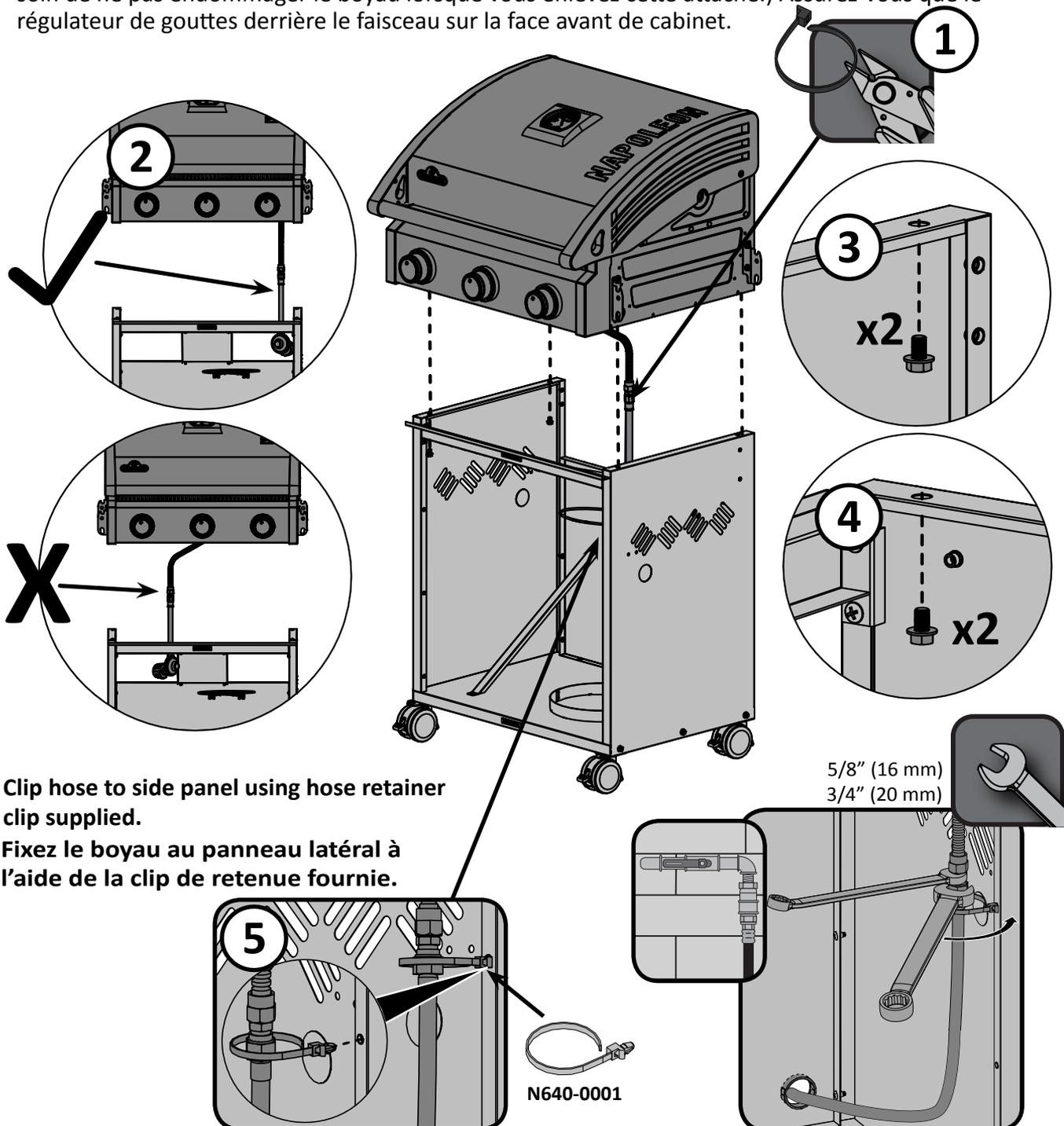
Clip hose to side panel using hose retainer clip supplied.
