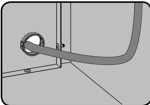
**Natural Gas Only – Improper Hose Connection**
