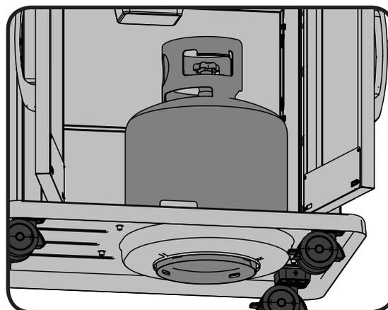
**Cylinder Connection:** Ensure the gas regulator hose is kink free. Remove the cap or plug from the cylinder fuel valve. Insert the black QCC1 regulator nipple onto the QCC1 fuel valve. Hand tighten clockwise. Do not use tools. Leak test all joints prior to using the grill. A leak test must be performed annually and each time a cylinder is hooked up or if a part of the gas system is replaced.
