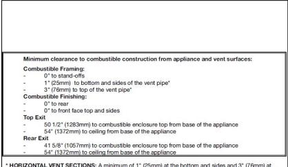
\* HORIZONTAL VENT SECTIONS: A minimum of 1" (25mm) at the bottom and sides and 3" (76mm) at the top of the vent pipe on all horizontal runs to combustibles is required. Use firestop spacer W010-1774 (supplied).
