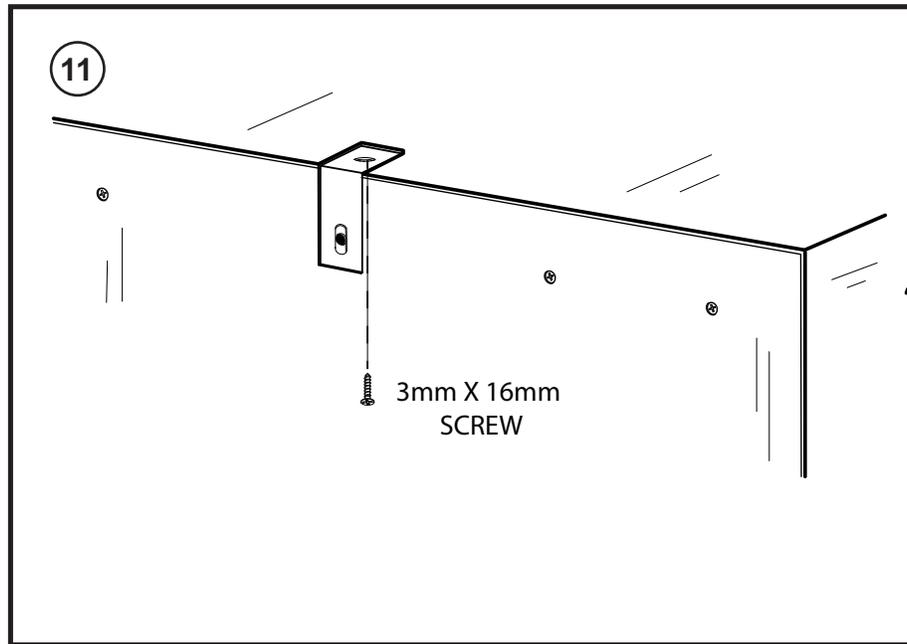
Secure top of bracket using screw from hardware kit.
