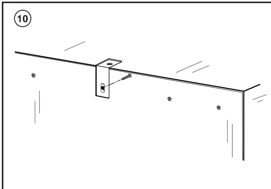
Secure bottom part of bracket using screw from step 9.
