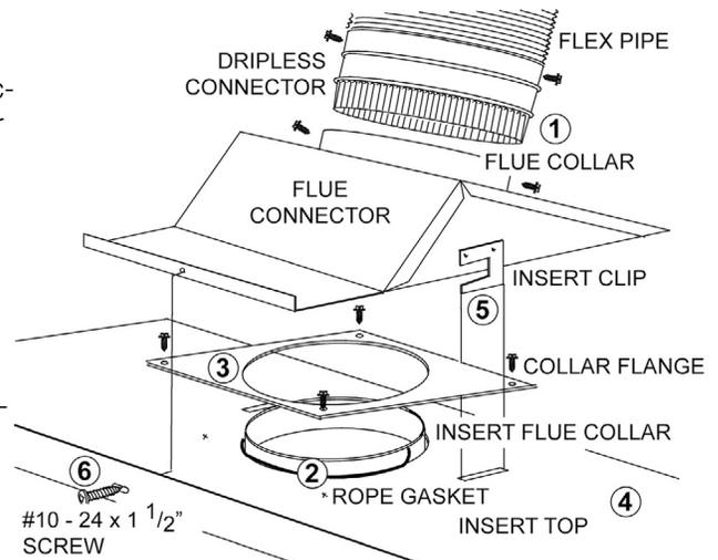
**NOTE: Check for a good seal between the insert top and the flue connector (by holding a flashlight up through the insert collar, etc.).**
