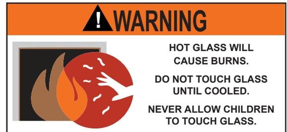
**DO NOT CLEAN GLASS WHEN HOT!** Clean the glass after the first 10 hours of operation with a recommended appliance glass cleaner. Thereafter clean as required.
