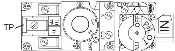
Disconnect the existing wires from terminals 1 and 3 (from the ON/OFF switch) and replace with the leads from the wall switch / millivolt thermostat.
