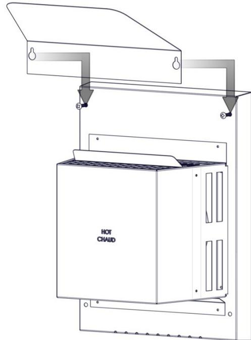
1. Loosen but **do not remove** top 2 screws from the terminal.
