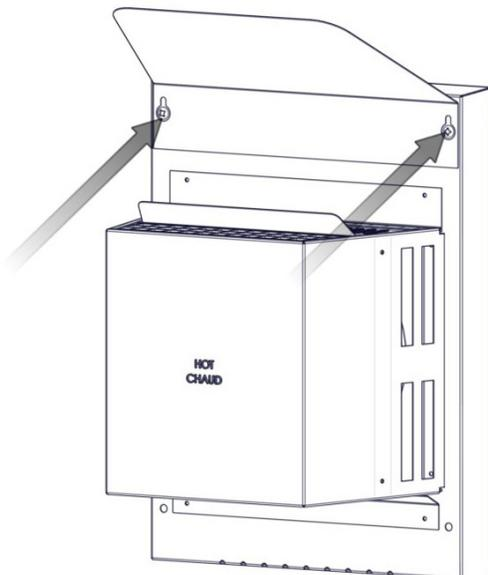
3. Tighten the two top screws to secure rain guard.
