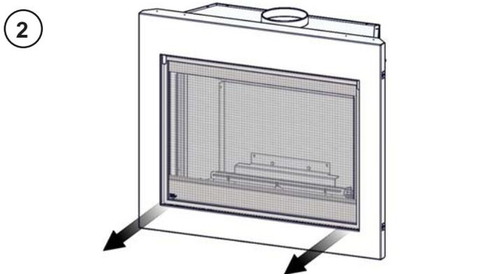
REMOVE THE SAFETY BARRIER ASSEMBLY BY PUSHING AGAINST THE BOTTOM CORNERS TO RELEASE THE TWO MAGNET CATCHES.
