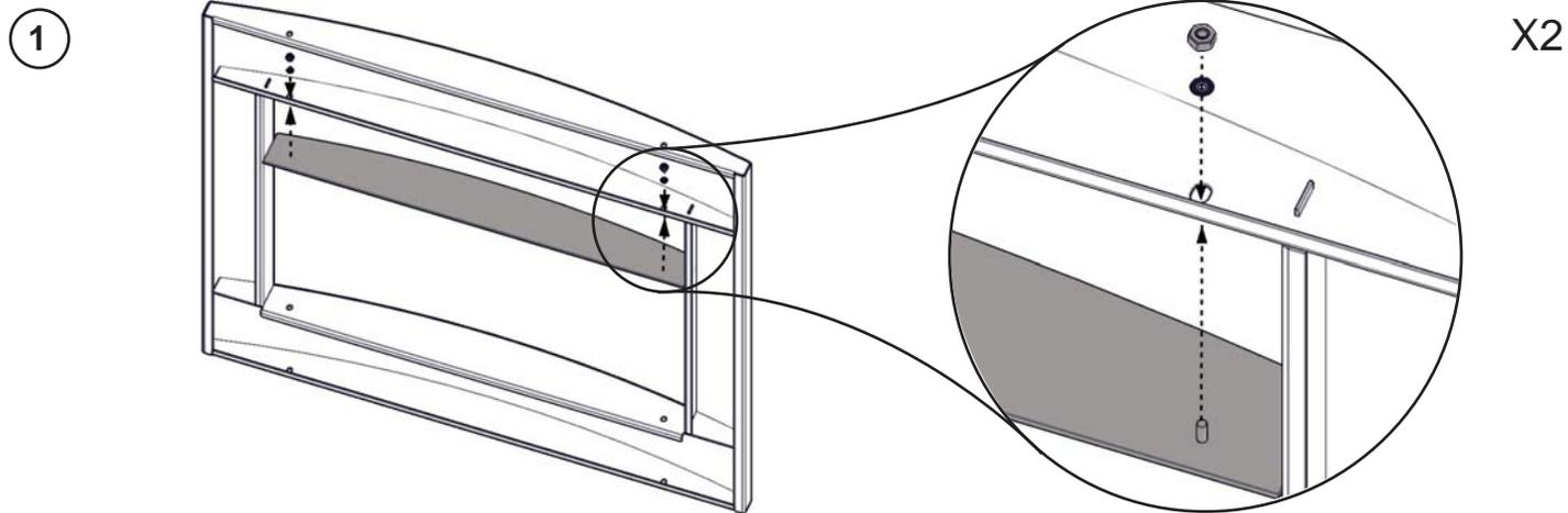
NOTE: DURING SHIPPING THE TRIM PIECES MAY MOVE, SIMPLY LOOSEN THE SECURING NUTS AND ADJUST.
